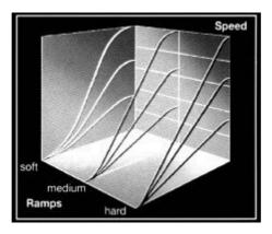
The start and stop ramps are programmed in our factory. Speed selector 1,2,3,4 and Super Jib on/off switch change the start and stop ramps according to the selected requirements.
