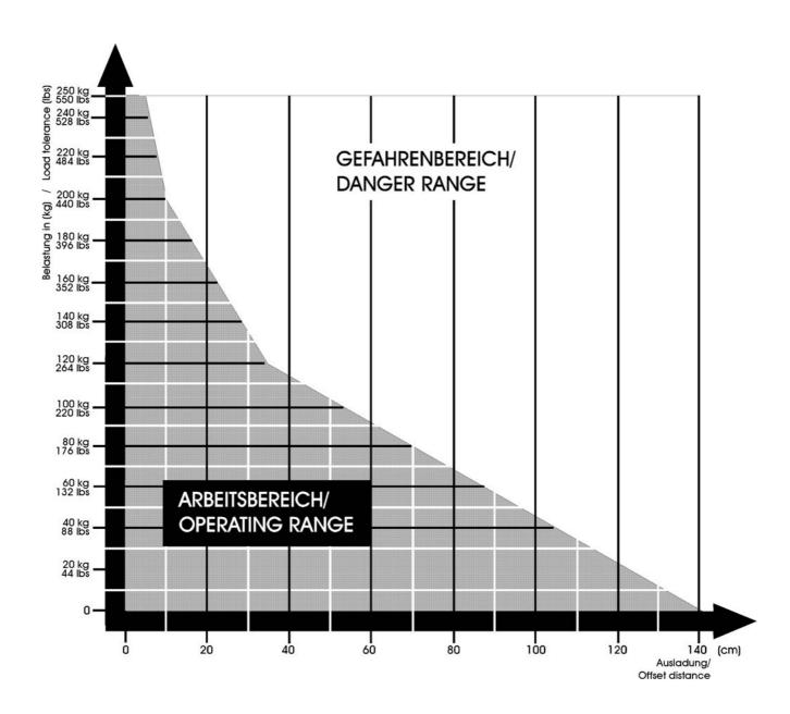
When using the Super Panther III with outriggers (e. g. outrigger III, U-Bangi), always use wide gauge wheel configuration for safety reasons (p. 12). The load tolerances diagram <u>must</u> be adhered to. maximum central column load: 250 kg / 550 lbs maximum offset distance: 140 cm
