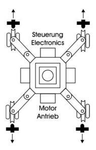
Align two wheels at a time using the wheel locking bar (wheels side by side) or the side locking bar (one wheel behind the other) and secure the pivot screws; then, the next two wheels, and so on.
