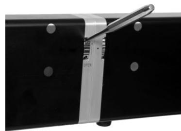
Once the dots are properly aligned, tighten the hammer bolt with the Swiss punch in the close direction, being careful not to over tighten. Warning, over-tightening may cause damage to the equipment.
