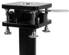
When assembling the jib arm on a base or dolly equipped with an Elemack boss, you should start with the leveling-head. Slide the leveling-head over the Elemack boss and turn the wheel clockwise in the leveling-head to secure the leveling-head onto the Elemack boss. It is advisable to use the punch which fits into the wheel.
