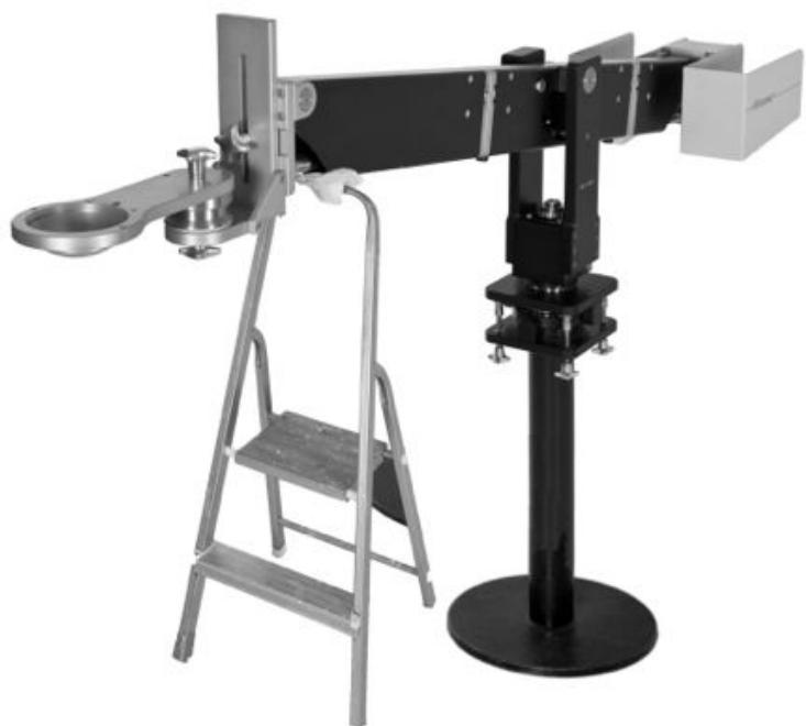
Balance the arm by putting some weight in the bucket, but maintain downward force on the support in the front end.
